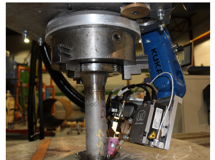
Standard chuck solution for easy assembling to the different work pieces
